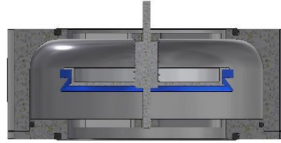
Overpressure valve when activated: open .
