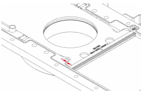
Fig. 87: Correctly inserted slide blade
